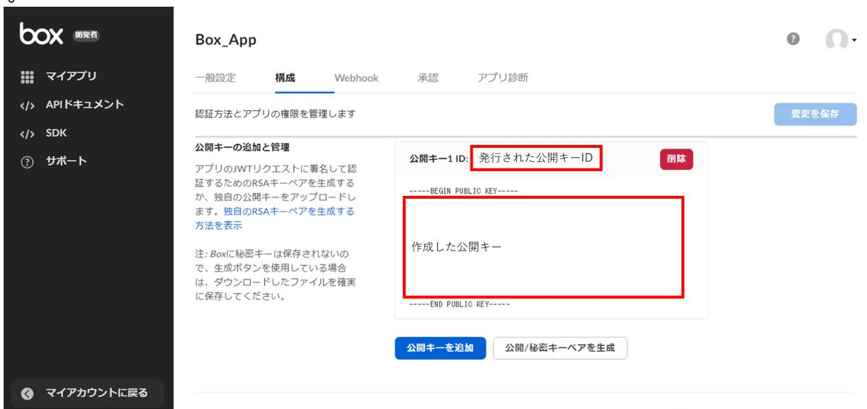
The screenshot shows the 'Box\_App' configuration page with the '公開キーの追加と管理' section expanded. The '公開キー-1 ID' field now contains '発行された公開キーID' and is highlighted with a red box. Below it, the '作成した公開キー' (Generated Public Key) is shown within a red-bordered box, flanked by '-----BEGIN PUBLIC KEY-----' and '-----END PUBLIC KEY-----'. The '公開/秘密キーペアを生成' button is now disabled.
