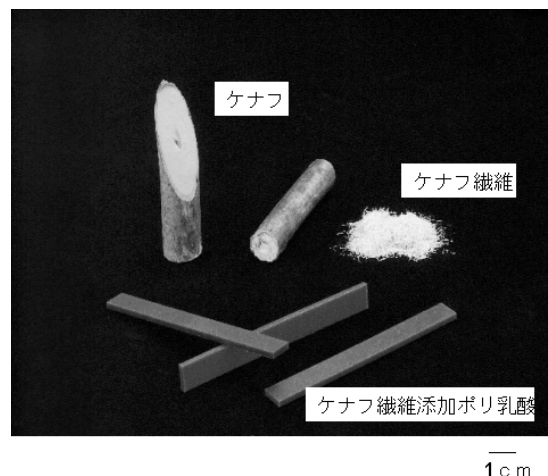
図2 ケナフ、ケナフ繊維、およびケナフ繊維添加ポリ乳酸(ケナフ繊維20wt%) Fig.2 Kenaf, kenaf fiber and kenaf fiber-reinforced bioplastic.
