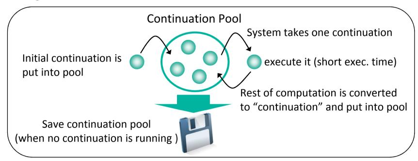
By saving the continuation pool, whole execution state can be saved, because it contains "rest of computation" as continuations
