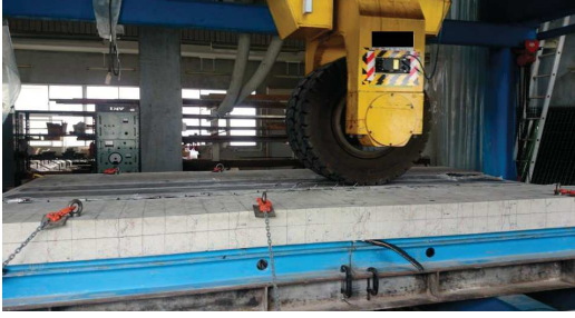
(a) Wheel loading setup on concrete bridge sample
