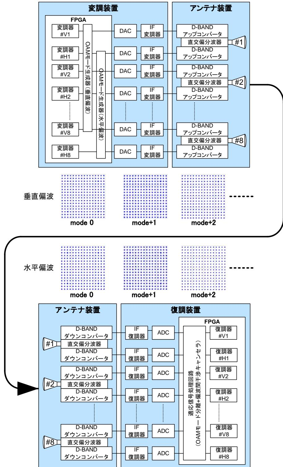
OAM mode and polarization multiplexing concept
