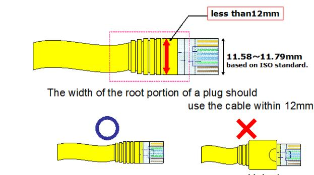
The width of the root portion of a plug should use the cable within 12mm.
