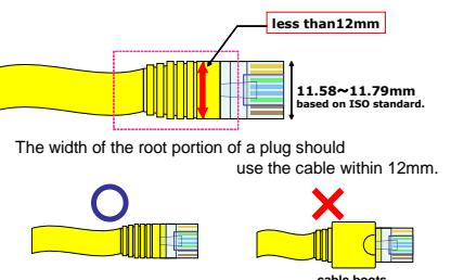
Refer to the left figure which does get used to use for the cable with boots (with a connector cover).
