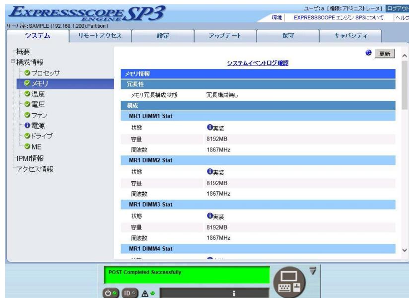
The screenshot shows the EXPRESSSCOPE SP3 interface with the 'メモリ情報' (Memory Information) section selected. The interface is divided into four main sections for MR1 DIMM1, MR1 DIMM2, MR1 DIMM3, and MR1 DIMM4. Each section contains the following data:
