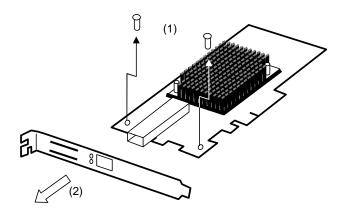
3. Install the low profile bracket to this product and tighten the two screws.
