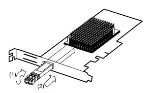
Replace the cover and components removed in item 2. (Take care not to conflict the SFP+ module with the cover edge.)
