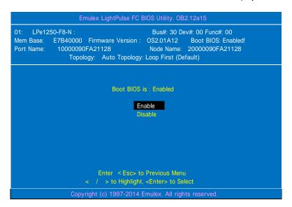
15> If any other ports of this product are connected to the Fibre Channel boot device, press <Esc> key to return to the adapter list and setting ports by the same steps from 4>.
