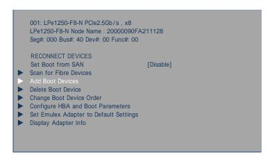
7> A screen appears displaying the discovered targets. Then select the Boot device and press <Enter>.
