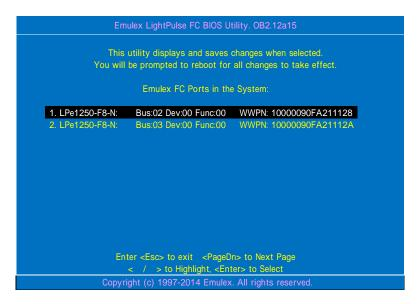
16>Now, you have made settings to start installing an operating system on your Fibre Channel device. Press <Esc> key to exit the menu. Then press <y> when this message is displayed, to reboot the computer and start installation.
