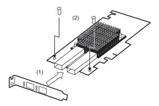
4. Replace the two SFP+ modules removed in item 1.
