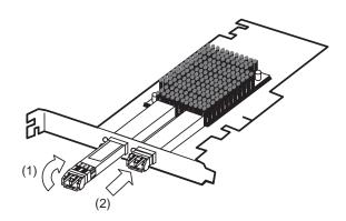
**6**. Replace the cover and components removed in item 2. (Take care not to conflict the SFP+ module with the cover edge.)
