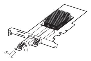
2. Remove the two screws and remove the bracket from this product.
