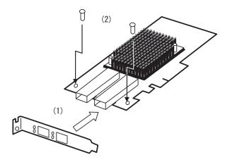
4. Replace the two SFP+ modules removed in item 1.
