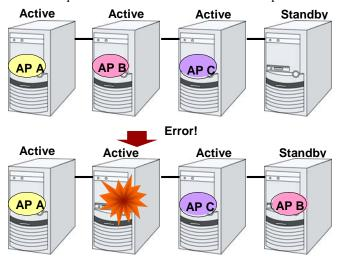
Figure 2-8 Node to Node configuration
