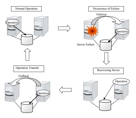
Figure 1-2: From occurrence of a failure to recovery
