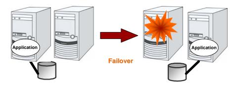
Figure 2-5 Uni-directional standby cluster system
