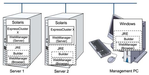
Figure 2-1 Software configuration of ExpressCluster
