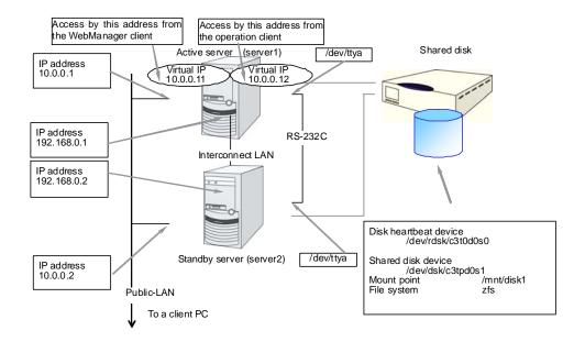
Figure 2-9 Sample of cluster environment when a shared disk is used
