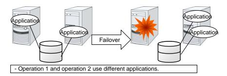
Figure 2-7 Different application multi directional standby cluster system
